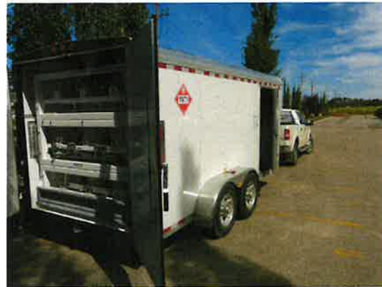
One of the three natural gas supply trailers. These can be used in the event of planned and unplanned outages.
